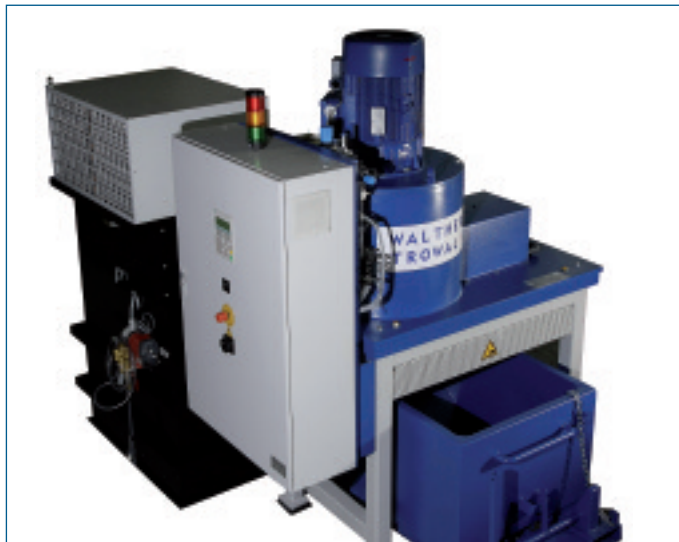
Peeling centrifuge ZA 04 with cooling system
