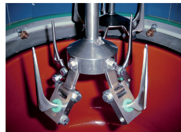
Drag finishing clamping device for hip implants
