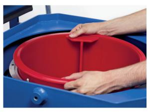
Simple exchange of sludge basket. No tools required!
