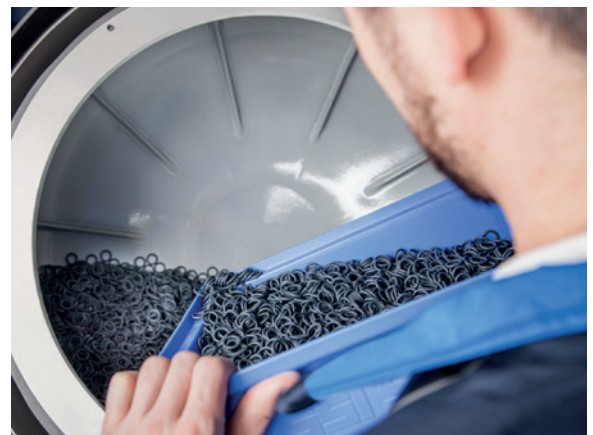
Loading of the drum with O-rings
