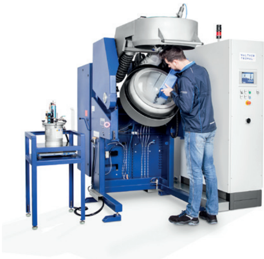
Loading of the drum with uncoated work pieces
