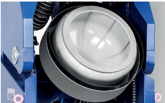
Drum with 3S lining
