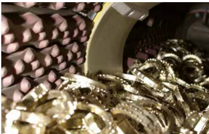
Geringer Turbinenabstand zum Strahlgut Short distance between turbines and parts
