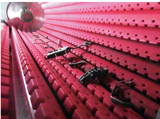
With the unique troughed belt transport system, the workpieces are gently passing through the machine
