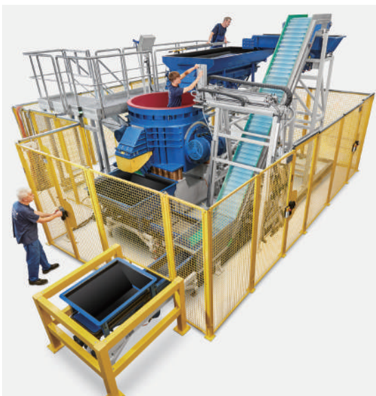
The workpiece is attached to the bottom of the processing bowl (center). The media is automatically transferred from the lower intermediate storage hopper to the upper loading hopper.
