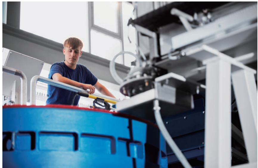
The MV 50 multivibrator runs fully automatically. All the operator has to do is to supervise the finishing process
