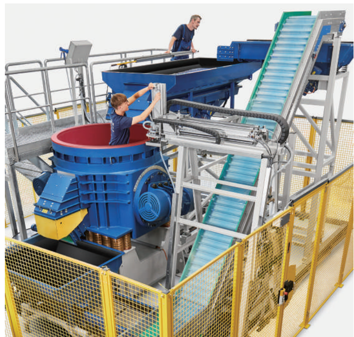
The processing bowl has an internal diameter of 1,600 mm
