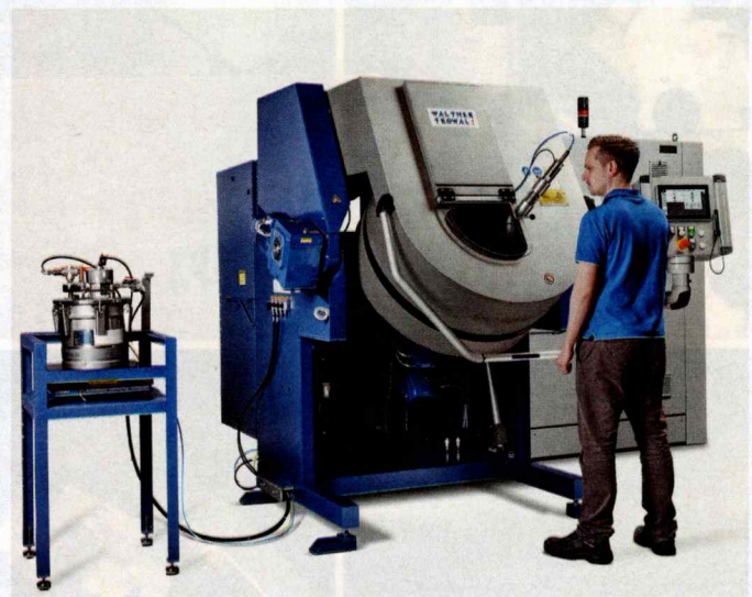
The new Rotamat R 100 system can coat plastic components with diameters of up to 300 mm
