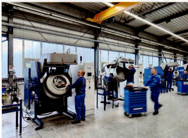
Final assembly of Rotamat coaters at Walther Trowal in Haan
