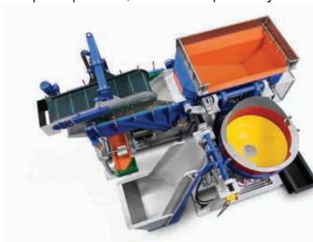
Walther Trowal supplies fully automatic systems, including workpiece loading & unloading. The photo shows a double batch system with magnetic separation
