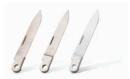
Knife blades before (left) and after (right) polishing in a TT machine. These workpieces require a particularly smooth, shiny surface
