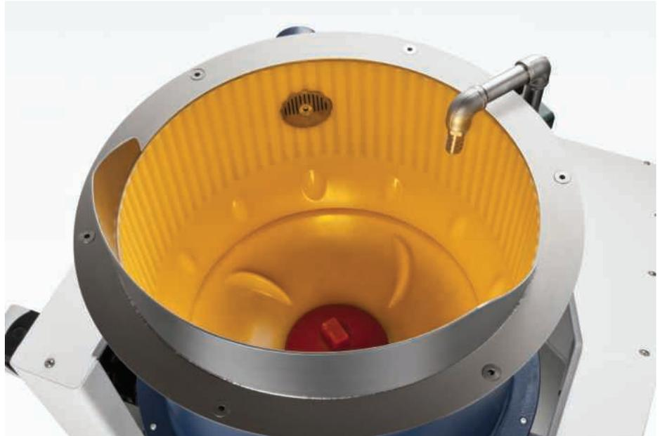
In the new TT centrifugal disk finishing machines, the gap (interface) between the (lower) rotating spindle and (upper) stationary work bowl is rinsed with process water
