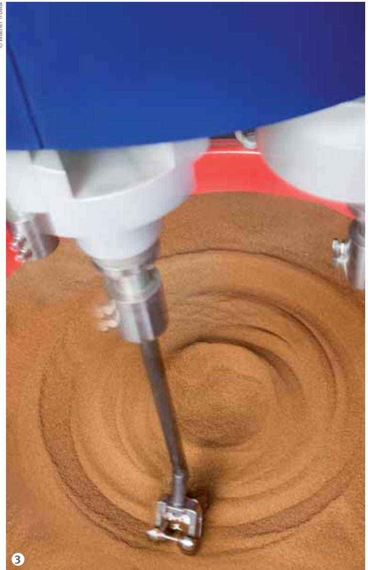
**Figure 3: A work piece shortly before being lowered into the grinding medium.**
