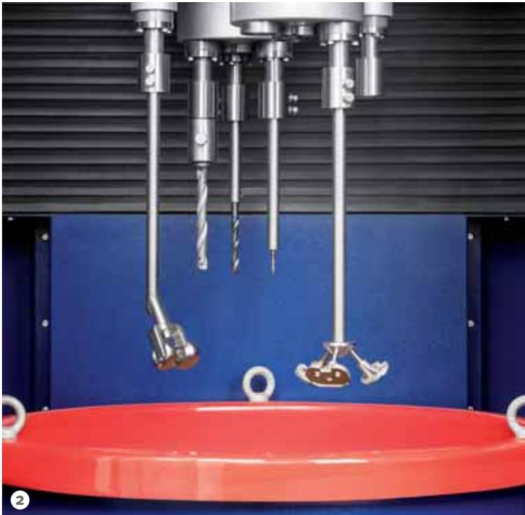
**Figure 2: The multi spindle heads allow attaching up to 18 parts. In this photo different parts were mounted onto one spindle head.**
