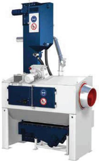
*The compact troughed belt continuous shot blast system THM 300/1 combines the small footprint of batch machines with the advantages of continuous feed operation. Photo: Walther Trowal*
