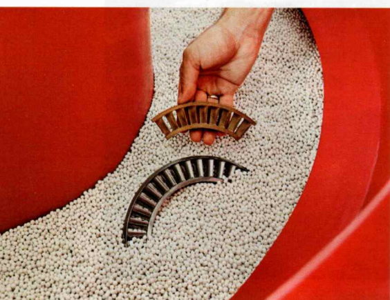
2/ A 3D printed blisk segment (top) and after the "Trowalizing" process
