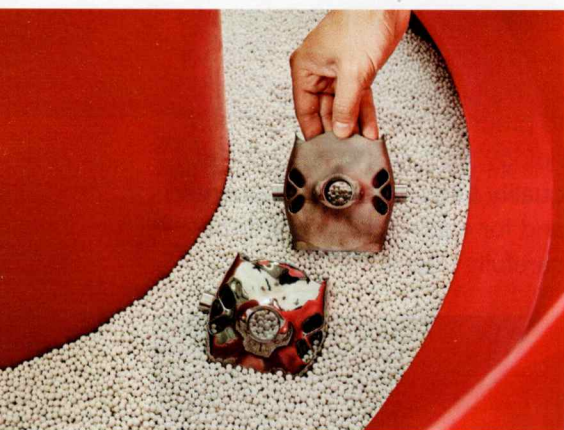
1/ A 3D printed gimbal frame before (top) and after the "Trowalizing" process (Pictures: Walther Trowal GmbH & Co. KG, Haan, Germany)
