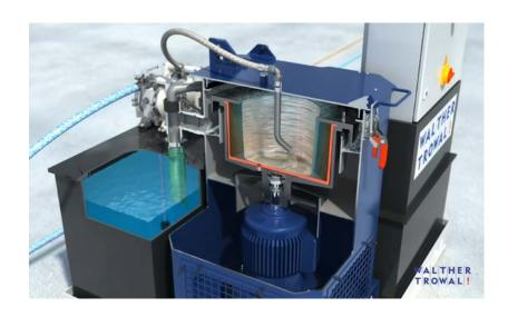
The centrifugal force of the rotating drum deposits the sludge on the wall of the drum insert. The cleaned process water is returned to the mass finishing equipment.
