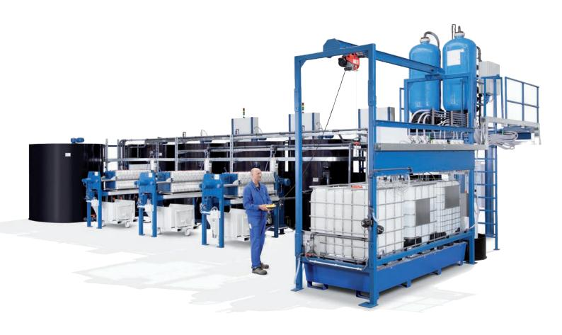
In PLC controlled flocculation systems up to 3,000 liters of process water can be cleaned per hour.
