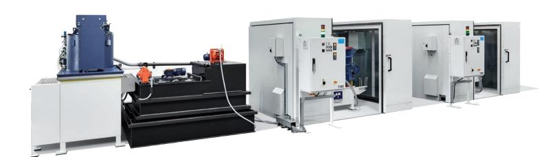
The contaminated process water coming from two rotary vibrators is cleaned and recycled back to the mass finishing operation.
