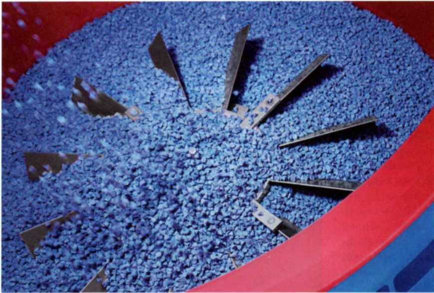
Plastic grinding media produce low surface roughness readings on the special shapes of blisks and the materials they are made of.
