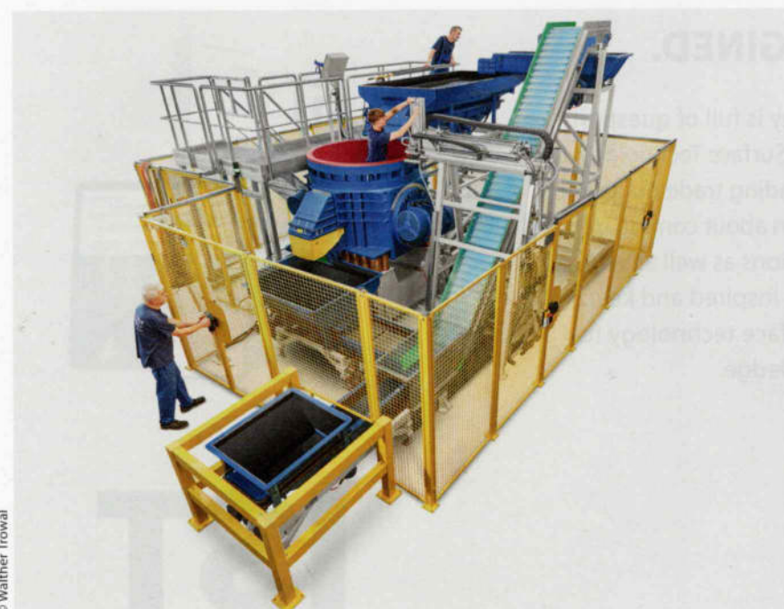
The work piece is firmly attached to the bottom of the processing bowl. The media is automatically transferred from the lower storage hopper to the upper loading hopper.
