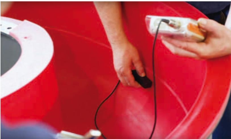
The thickness of the new wear lining is measured and documented
