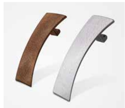
A 3D printed clip before (left) and after the “trowalizing” process
