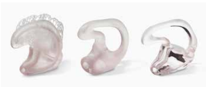
A 3D printed ear piece for a hearing aid before (left), surface smoothing (center) and after polishing
