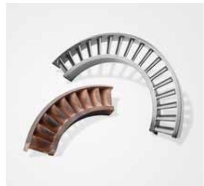
A 3D printed blisk segment before (left) and after the “trowalizing” process
