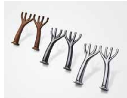
A 3D printed nozzle before (left), after surface grinding (center) and after polishing
