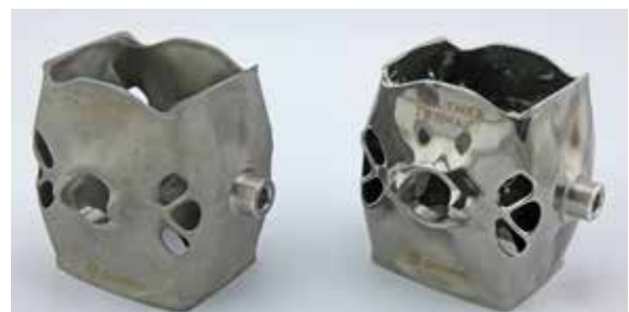
A 3D printed gimble frame before (left) and after the “trowalizing” process
