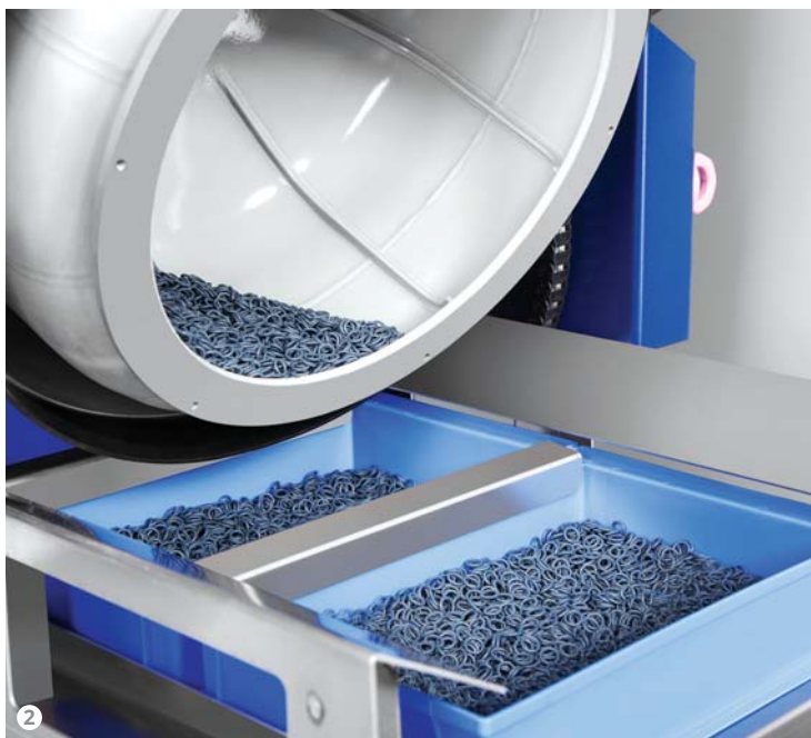
Figure 2: With a diameter of only 600 mm the drum is adjustable to different work piece geometries and allows the complete, optimum coverage by the spray nozzles.
