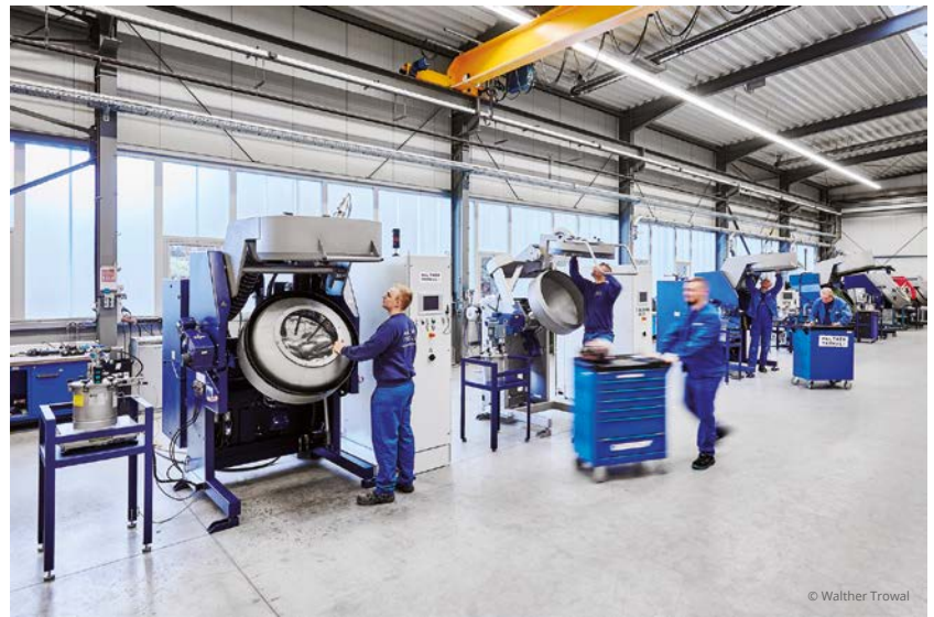
The new Rotamat R 100 allows the coating of components with diameters of up to 300 mm. On the right, Rotamat coaters in the final assembly stage at Walther Trowal in Haan.
