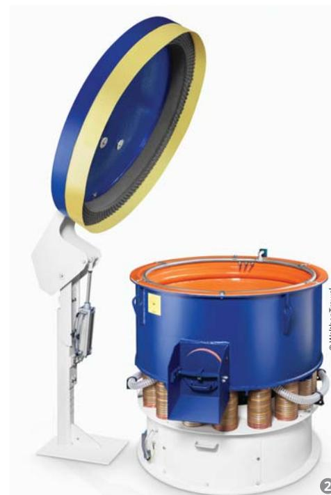
Figure 2: In the "CM" rotary vibrator work pieces with a diameter of up to 980 mm can be processed. During the finishing process itself the work bowl is covered with a noise absorbing lid.
