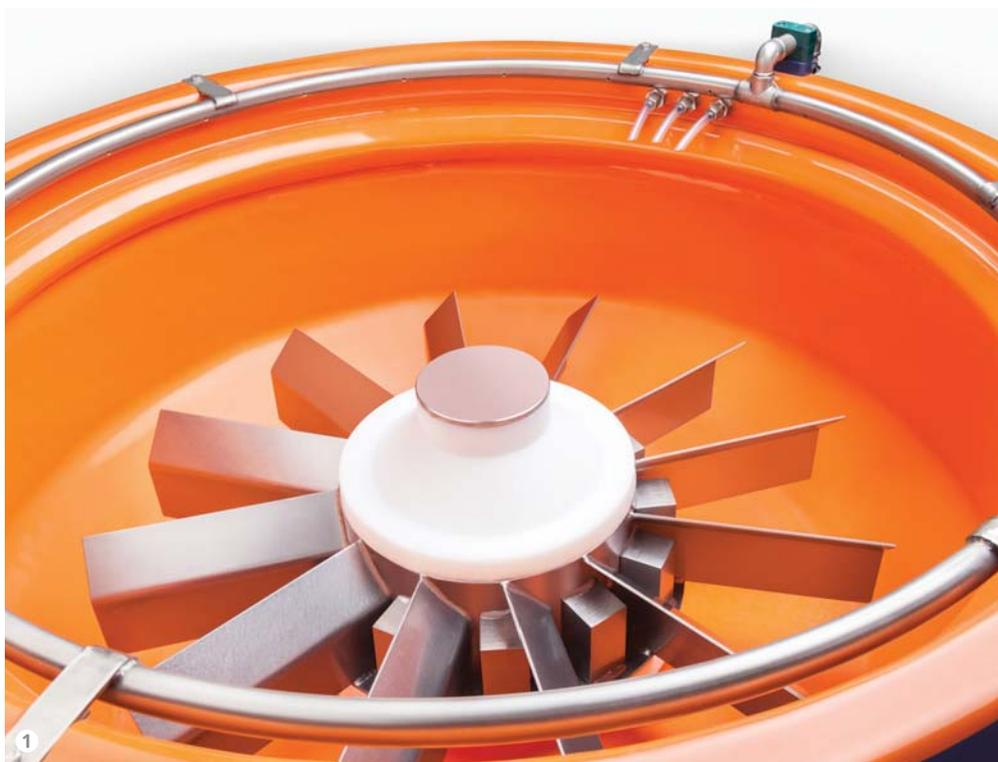
Figure 1: The work bowl of the "CM" rotary vibrator. The shown work piece is a dummy.
