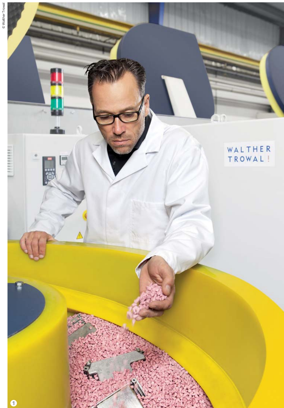
Figure 1: The mass finishing technology can be used for surface grinding, smoothing and polishing as well as for deburring of castings.
