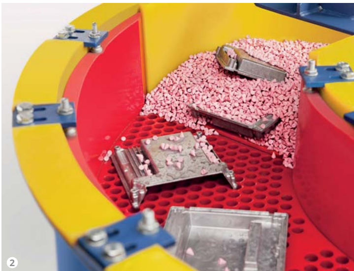
Figure 2: The processing media is safely removed during the separation phase, even from "cup-shaped" parts.
