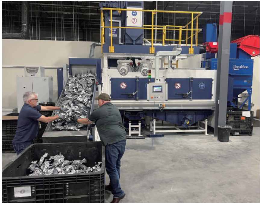
A THM 400 shot blast machine in the TTC test and training center in Grand Rapids/USA is loaded with aluminum die-castings for the automobile industry
