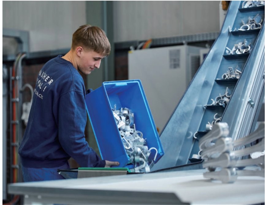
Typical applications for the THM shot blast machines are forged chassis components made from aluminum like transverse links, swivel bearings or steering knuckles. They are equally suitable for high volumes of mass-produced aluminum die-castings.
