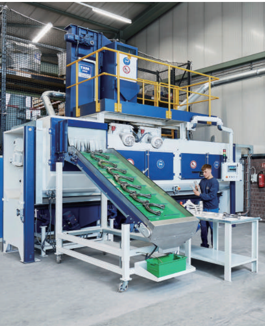
A THM 500 troughed belt continuous flow shot blast machine in the Trowal test and training center in Haan/ Germany
