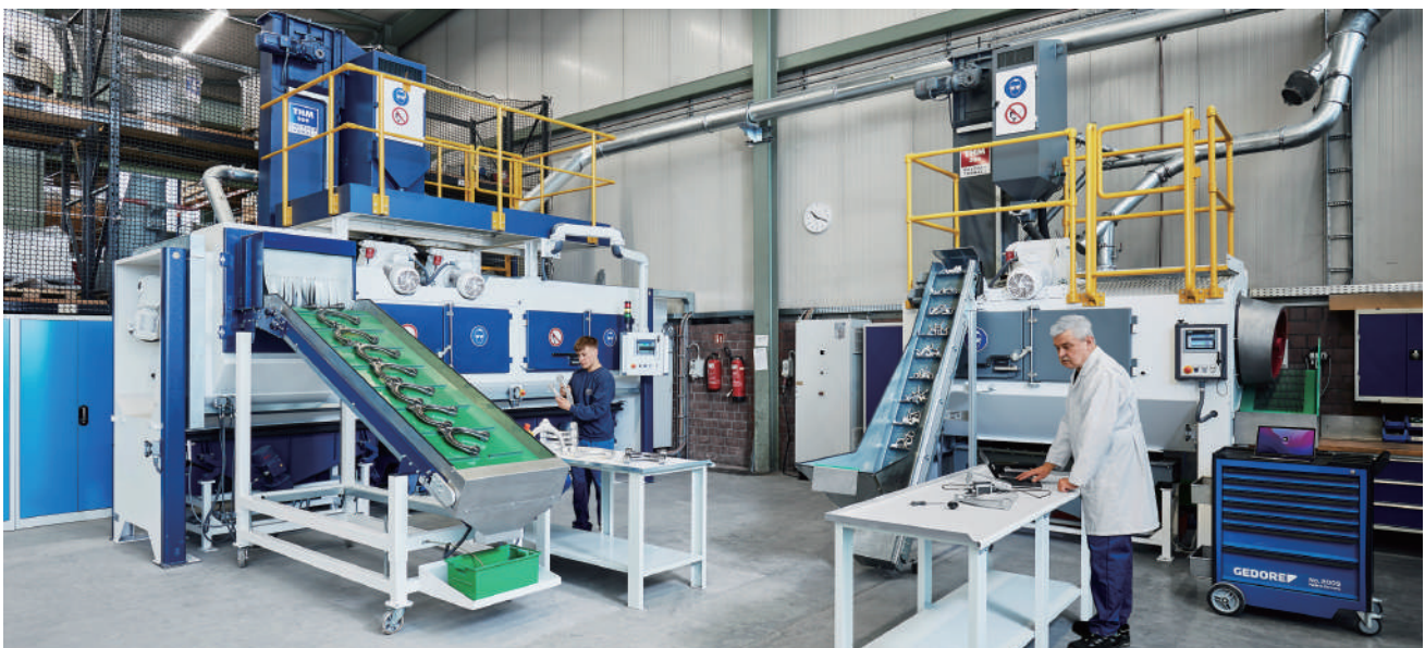
The Trowal test and training center is equipped with several THM shot blast machines that can be used for processing trials with the customers' work pieces.
